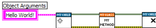
Creating a child class object, calling parent method and closing the child object
